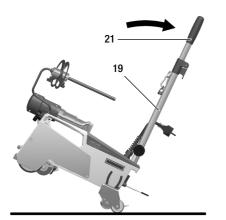
To position the hot-air welder, press the **guide bar** (19, 21) and then roll the UNIFLOOR 500 this way into the desired welding position.
