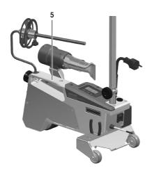
To manually raise the semi-automatic hot-air welder, use the **carrying handle (5).**
