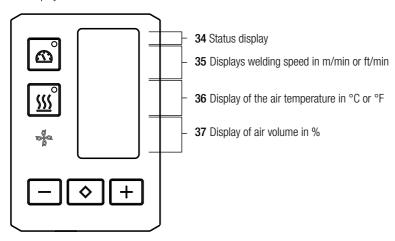
During operation, the setpoints of the welding parameters (drive in m/min or ft/min, temperature in degrees Celsius or Fahrenheit), air volume in percent and, if applicable, information notes are displayed.
