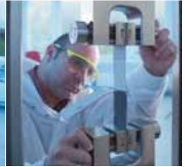
Peel testing with welded plastic specimens.
