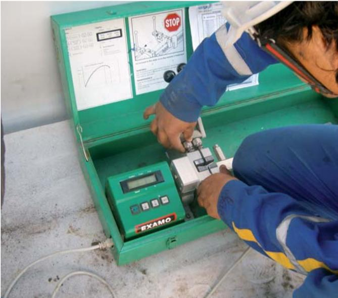
*The tensile tester EXAMO for checking the relevant welding parameters.*
